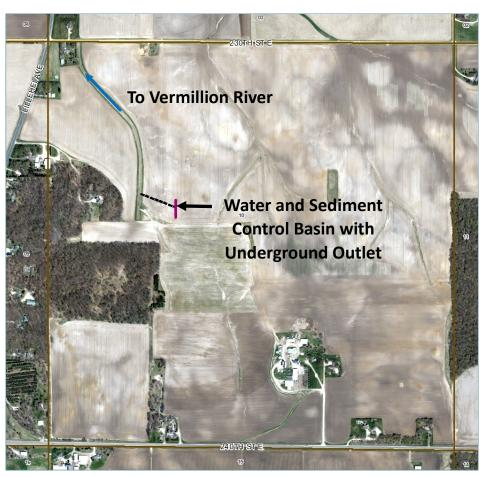
**PROJECT:** Surface water runoff is causing erosion in the field. The project includes the installation of a new water and sediment control basin that will outlet into an existing waterway.
