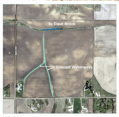
**PROJECT:** The existing grassed waterways are beyond their functional lifespan and surface water runoff that cannot be handled by the waterways is causing gully erosion in the field. The waterways will be reconstructed to adequately convey runoff.
