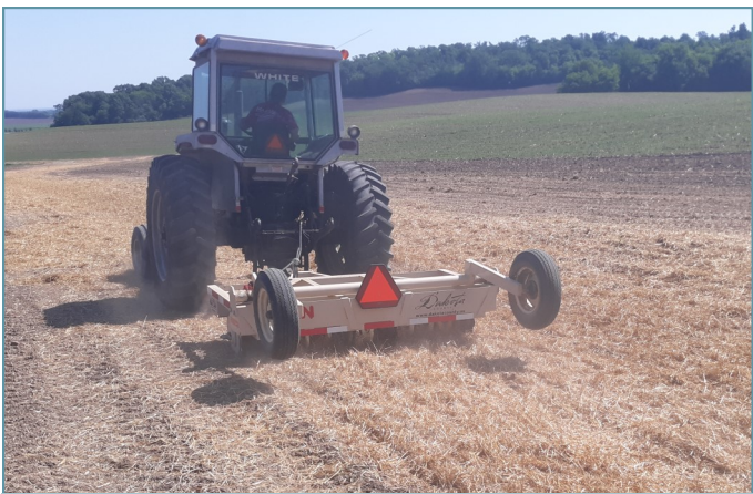
Straw mulch was anchored using a crimper to keep mulch in place.
