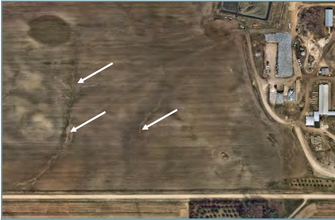
Surface water runoff had caused gullies to form in the field. Basins were designed to capture and manage runoff.
