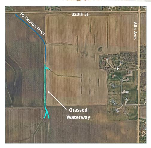
**PROJECT:** 1,500 linear feet of grassed waterway will be reconstructed. The existing waterway has exceeded its functional lifespan and surface water runoff is flowing through the field and causing erosion. The waterway is located along the property line and reconstruction is a joint project between the landowners.
