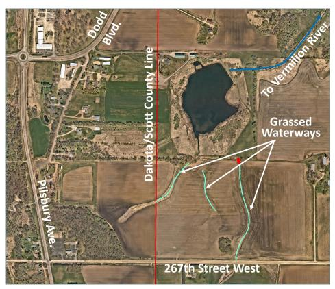
**PROJECT:** Surface water runoff is causing gully erosion in a concentrated flow channel and within two existing waterways that are beyond their functional lifespan. The project will install three grassed waterways to adequately convey the runoff and reduce future erosion.
