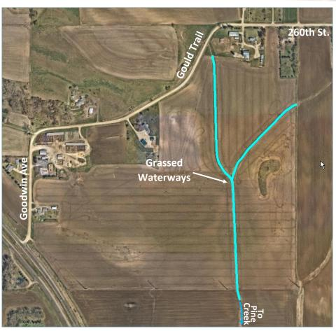
**PROJECT:** The existing waterways have exceeded their functional lifespan and surface water runoff is flowing through the field and causing erosion. The waterways will be reconstructed to adequately convey runoff and minimize future erosion.
