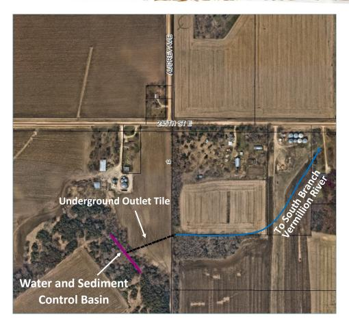
**PROJECT:** Surface water runoff is causing gullies to form in the field. A water and sediment control basin will be constructed to capture runoff, release runoff through an underground tile that discharges to a stabilized outlet, and reduce future erosion.
