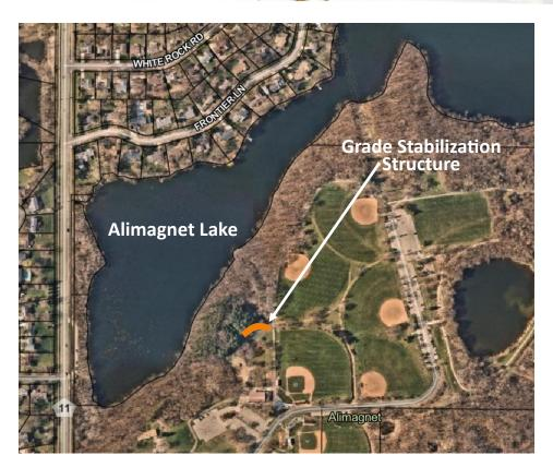
**PROJECT:** The City of Burnsville will install a grade stabilization structure (detention basin) at Alimagnet Park. The project will intercept and slow the flow of stormwater that is causing gully erosion near the shore of Alimagnet Lake.
