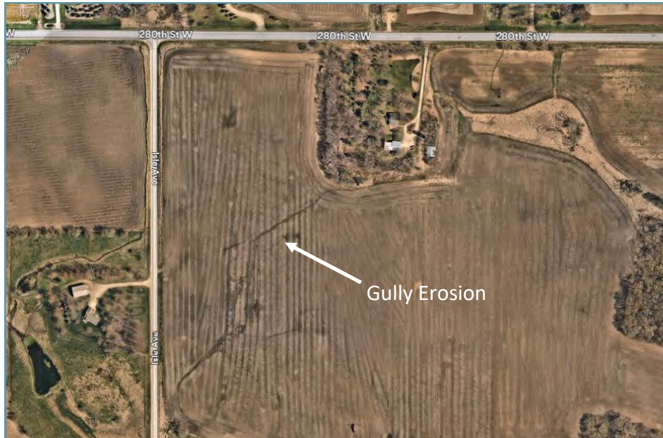
Aerial photo of project area prior to project. Gullies occurred annually in the agricultural field due to concentrated surface water runoff.
